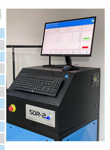
This model can test 2 injectors at the same time (2 el.mag/1 piezo)
