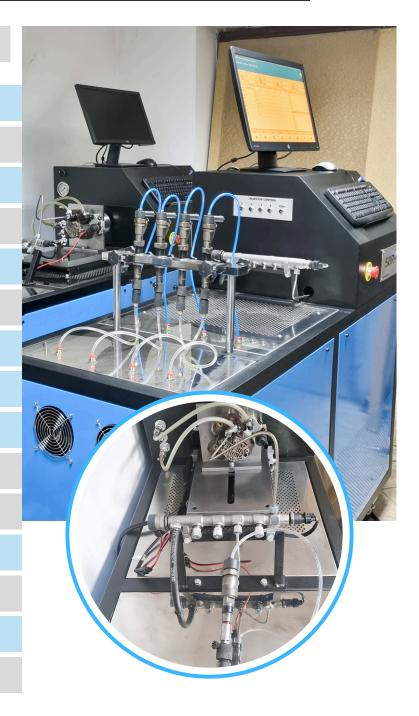
IPR series can test CR pumps and 1 or more injectors
