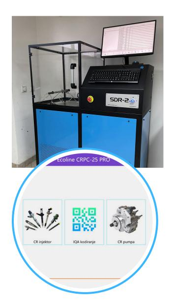
This model is for specialized injector repair shops. In addition to testing it can generate new code (after injector is repaired)
