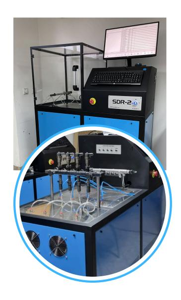
This model can test 4 injectors at the same time (4 el.mag/1 piezo)
