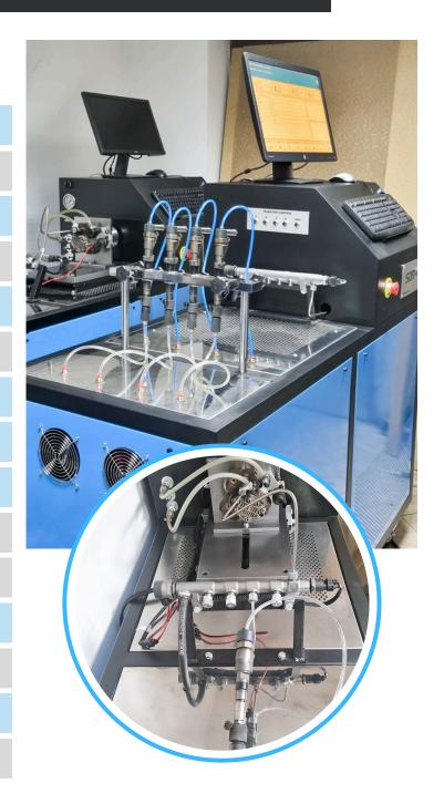
This model is for specialized injector repair shops. In addition to testing it can generate new code (after injector is repaired)
